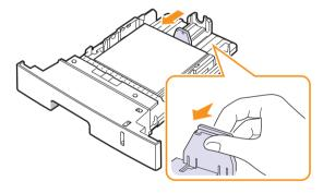
Squeeze the paper width guides, as shown and slide them to the stack of paper until it lightly touches the side of the stack.
